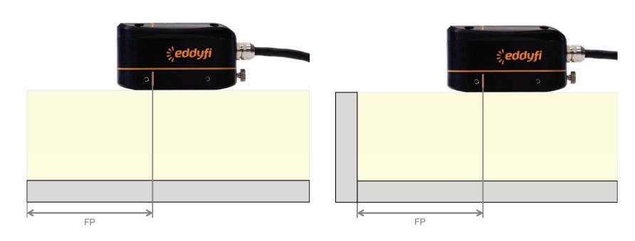
FP<sub>o</sub> is the footprint at a **liftoff of zero**. For each probe, FP<sub>o</sub> is:
